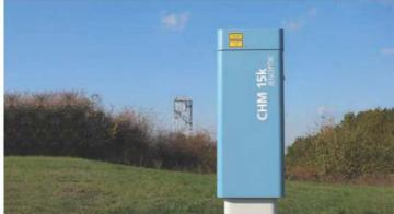
The "NIMBUS" series is the second generation of proven CHM 15k ceilometers measuring aerosol height profiles using the LIDAR technique. They determine cloud base heights, penetration depths, mixing layer height and vertical visibility. Within their operating range of up to 15 kilometers (50 000 feet), they reliably detect multiple cloud layers and cirrus clouds. The "NIMBUS" series is equipped with an integrated controller offering improved range resolution and a comfortable web interface.
