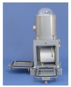
A further and quite remarkable improvement is the new shape of the casing. With model 58c, the whole casing had to be taken off for a change of charts. In the new instrument, however, the drum has been installed in the lower, cubic part of the casing, while the bimetallic strips are arranged at the top of its upper, cylindrical part. The two parts of the casing are separated from one another by a horizontal wall, which offers the following essential advantages:
