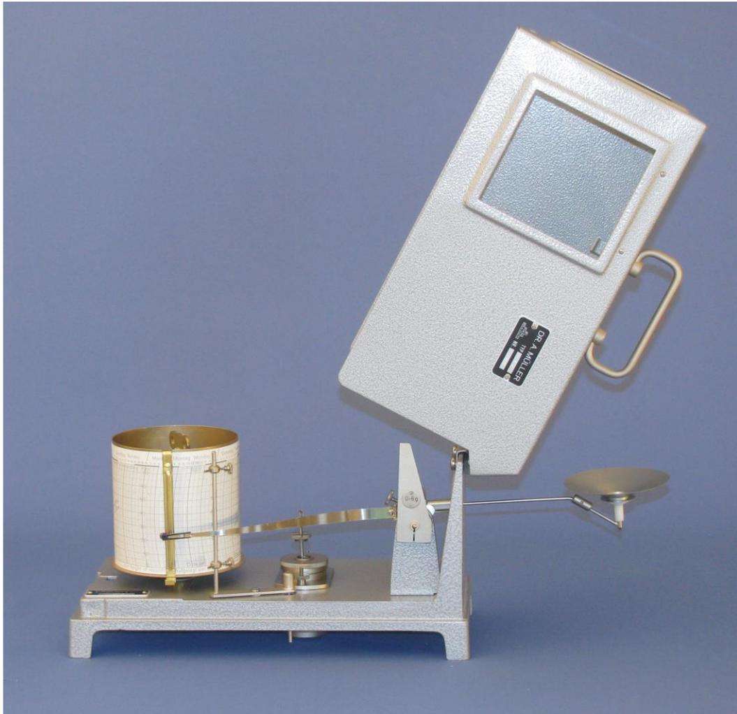
The dew recorder registers the precipitation of dew, the quantity of which depends on the temperature, the humidity, and the movement of the air, as well as on the temperature of the receiving surface which itself is influenced by its own radiation. A horizontally arranged plate of metallic serves as collector. The size of its effective surface which includes upper and lower side amounts to 110 cm<sup>2</sup>.
