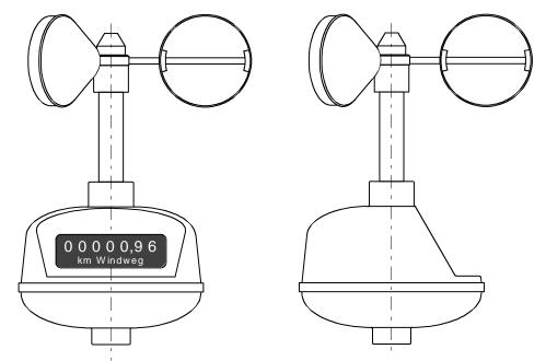
The counter maximally counts up to 99,999.99 km of wind run. One unit of the last reel of figures corresponds to a wind run of 10 m. In order to fasten the counter anemometer on a steel tube, the hub of the lower part of the casings has an inner diameter of R 1/2". The anemometer is executed in a splash proof kind of way, and the surfaces are protected by an exceptionally weather-resistant light-grey hammertone finish.
