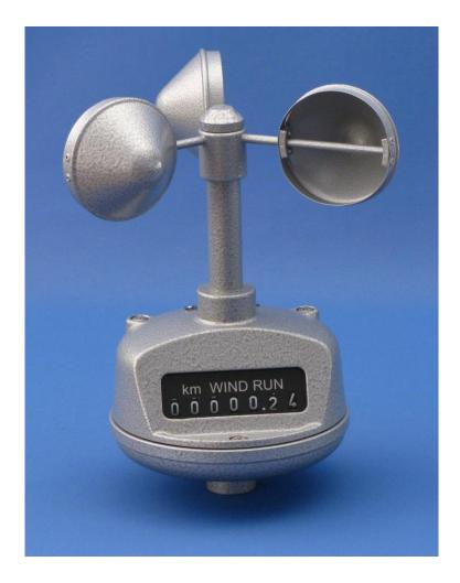
Large Weatherproof Counter Anemometer 91ge is used in wind measurement in the free atmosphere, for whatever periods of time. It is meant for continuous operation in the open and is used to measure air currents in heights from appr. 1.5 m on downwards. Actual position of the counter may be read directly, through the upwards, i. e., at an angle of 30° inclined window. The height of the figures is 8 mm.
