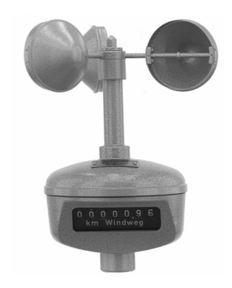
Large Weatherproof Counter Anemometer 91g is used in wind measurement in the free atmosphere, for whatever periods of time. It is meant for continuous operation in the open and is used to measure air currents in heights from appr. 2 m on upwards. Actual position of the counter may be read either directly, through the downwards, i. e., at an angle of 30° inclined window or, at greater heights of installation, with the aid of binoculars. The height of the figures is 8 mm.
