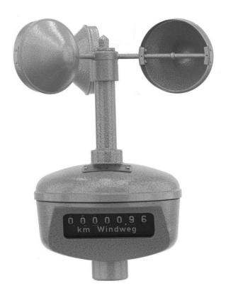
Large Weatherproof Counter Anemometer 91g is used in wind measurement in the free atmosphere, for whatever periods of time. It is meant for continuous operation in the open and is used to measure air currents in heights from appr. 2 m on upwards. Actual position of the counter may be read either directly, through the downwards, i. e., at an angle of 30° inclined window or, at greater heights of installation, with the aid of binoculars. The height of the figures is 8 mm.
