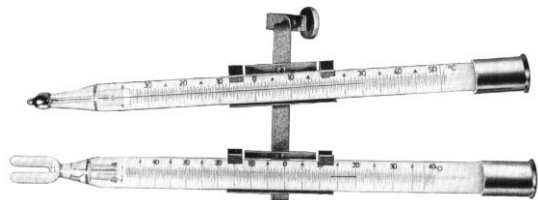
Fig. 3 Maximum and Minimum Thermometers with Support T23 UG14
